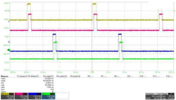
Figura 4: PG-1074 model: four channel synchronized with delay between 100ps and 1 ns
