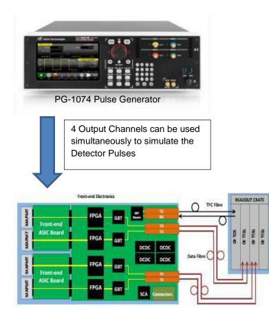
Figure 3: Principle scheme of read out chain: the Pulse Generator PG-1000 substitute the the photomultiplier and the charge amplifier during the preliminary test.
