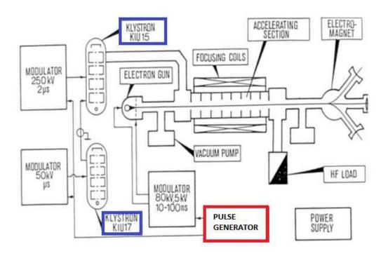
Figure 2 Example of complex system, where a Pulse Generator PG-1000 can synchronize two klystrons
