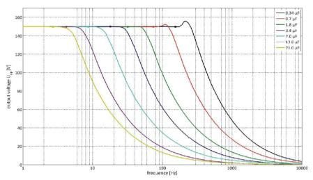
The diagram shows the typical frequency of the NV 40/3 series which can be reached as a function of the capacitance of the piezoelectric actuator and the driving voltage by an output current of 40mA.
