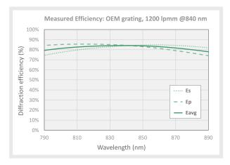
We measure every VPH transmission grating to ensure exceptional 1st order diffraction efficiency uniformity over the specified operating band. Not all vendors do!
